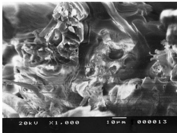
Figure 11 The intimate bonding between the fiber bundle and the resin in 0.2% treated composites.
